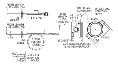
The Series TE Duct and Immersion Building Automation Temperature Sensors can be used to monitor air or water temperature throughout a building management system or an air handler unit. Duct or immersion options available with or without an
